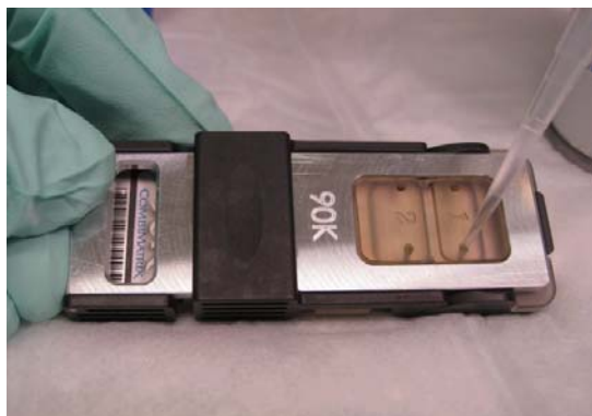
Figure 3. Ready to use CustomArray™ 2x40K assembled with the Hybridization Cap in the Hybridization Clamp. To add/remove solutions, hold the assembled microarray at a 45 degree angle and pipet through the lower portals of hybridization chambers.
