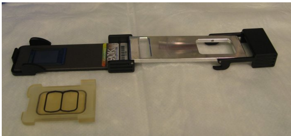
Figure 1. Placement of the CustomArray™ 2x40K in the Hybridization Clamp.
