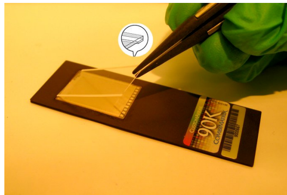
Figure 4. A CombiMatrix microarray with LifterSlip™ coverslip
