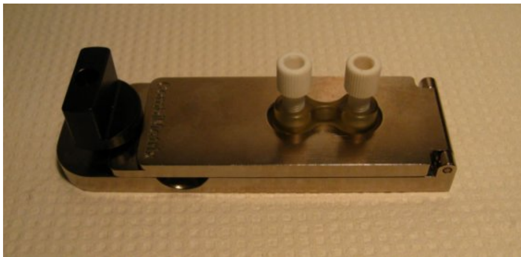
Figure 4. Assembly of the Stripping Clamp with the screw plugs.
