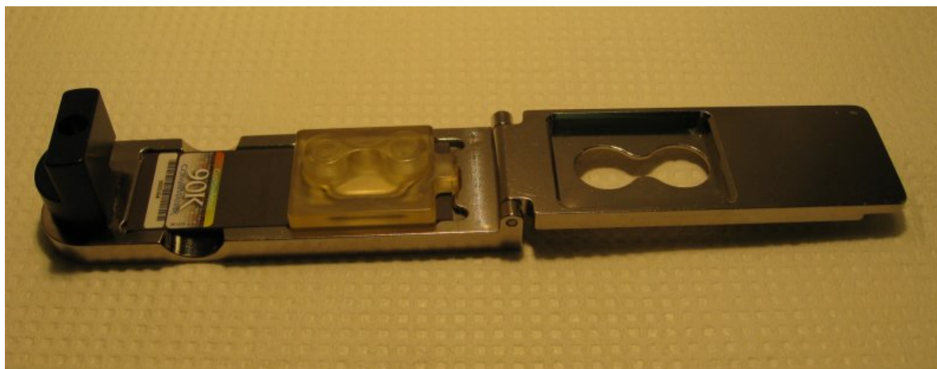
Figure 2. Position of the Stripping Cap over the microarray in the CustomArray™ Stripping Clamp.
