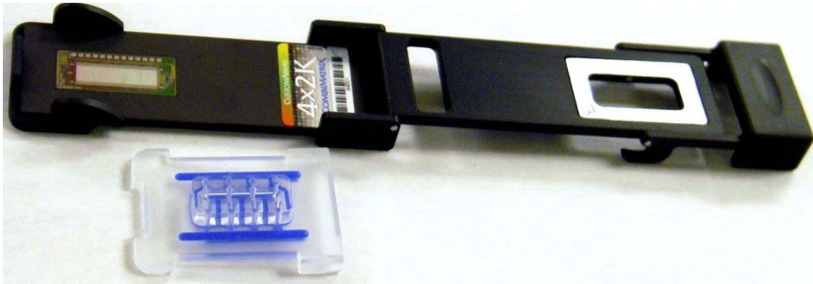
Figure 2. Placement of the CombiMatrix 4X2K microarray in the Hybridization Clamp.
