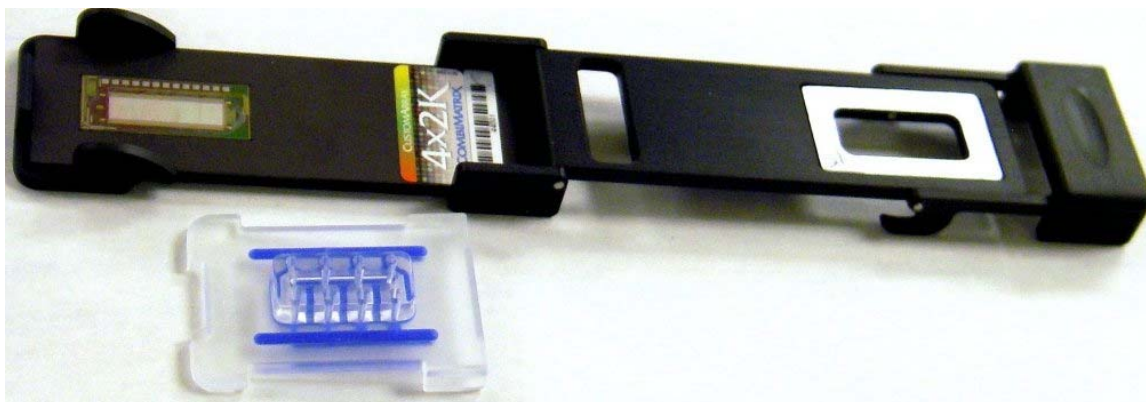
Figure 2. Placement of the CustomArray™ 4X2K in the Hybridization Clamp.
