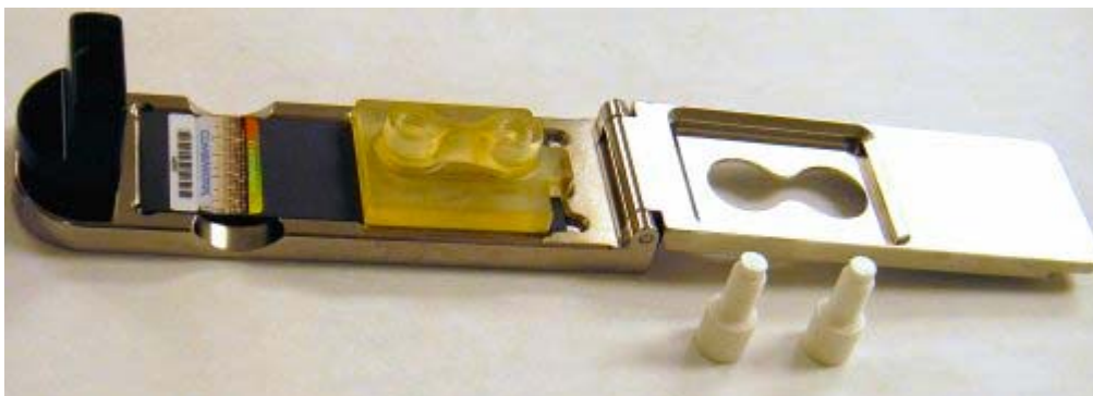
Figure 2. Position of the Stripping Cap over the microarray in the CustomArray™ Stripping Clamp.
