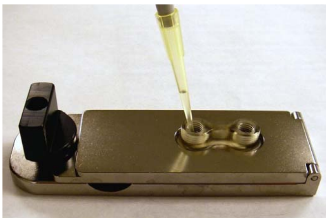
Figure 3. Pipetting of solutions into the assembled CustomArray™ Stripping Clamp.
